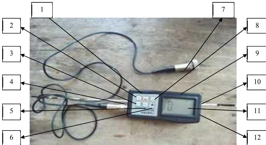
Gambar 3.11 *Vibrometer Handle*
