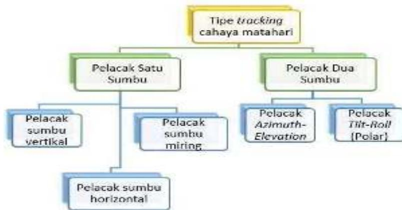
**Gambar 2.12 Tipe solartracking berdasarkan sumbu putaran
