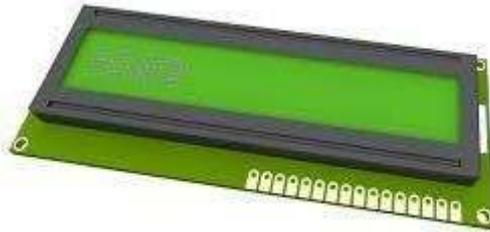
**Gambar 2.19 Liquid Crystal Display (LCD)**
