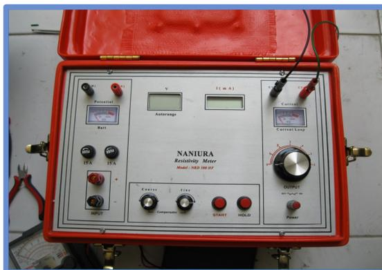
**Gambar 10.2:** Resistivity Meter Naniura NRD 300Hf (Ibnu Rois, 2020)
