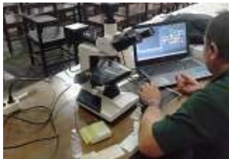
Gambar 3.34 Proses Pengukuran Diameter Serat
