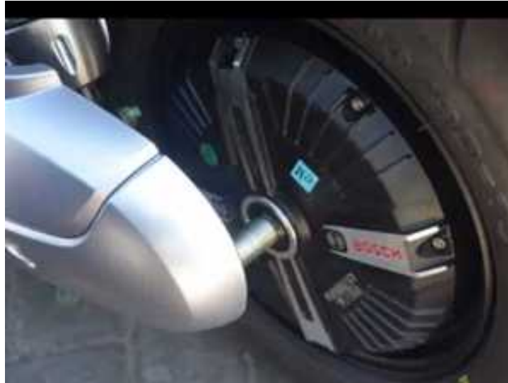
Gambar : 2.2 Jenis Motor Listrik Merek Bosch (Germany).
