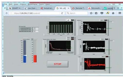
Figure 8. Dashboard Web control application a DC motor
