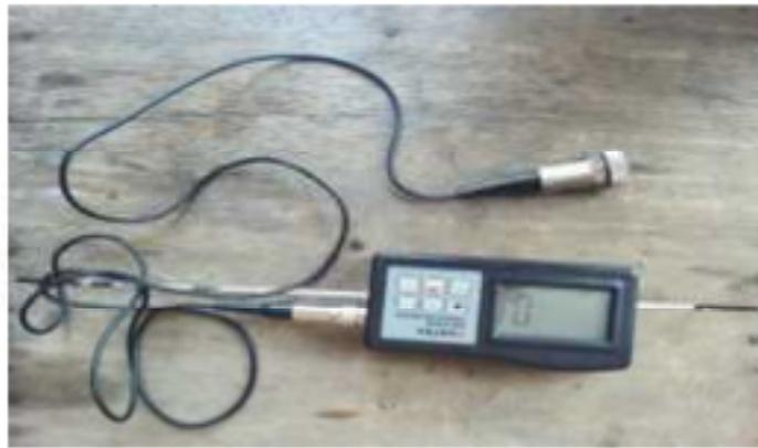
Gambar 3.1 Vibrometer Handheld
