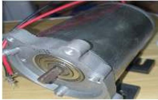
**Gambar 3.6 Generator DC 30 watt**
