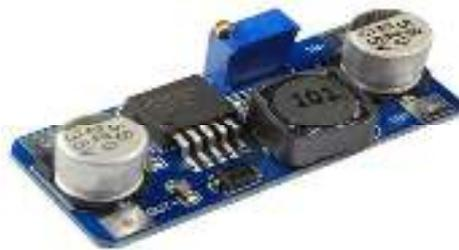
**Gambar 3.7 Step Up Converter Booster DC-DC type XL 6009**
