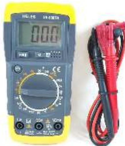
Gambar 3.3 Multimeter
