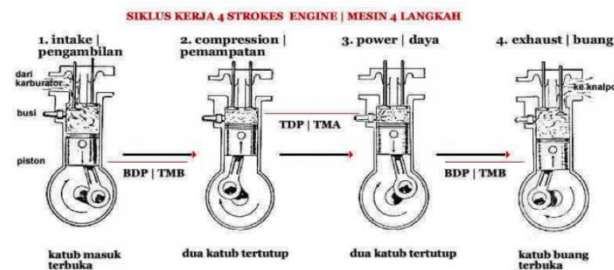
Gambar 2.2 Proses Kerja Mesin 4 Tak (Sumber: https://fastnlow.net )
