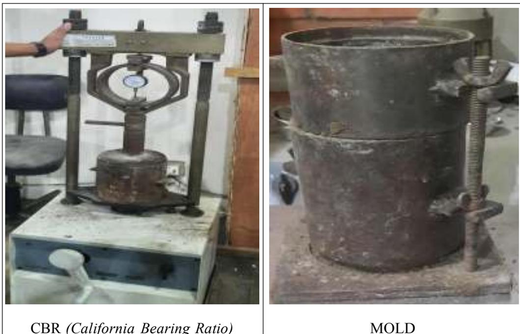
Gambar 3.11 Alat Pengujian CBR (*California Bearing Ratio*)
