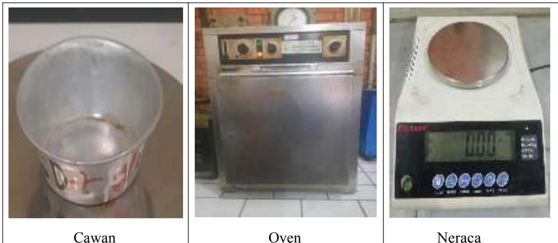
Gambar 3.4 Alat Percobaan Kadar Air
