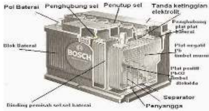
Gambar 2.19 Starting Battery
