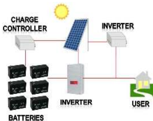
Gambar 2.2 Sistem PLTS Off Grid
