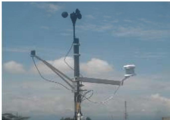
Gambar 3.6 Hobo Microstation Data Logger
